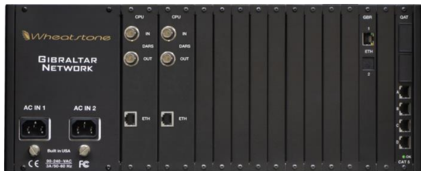
Figure 2-5 Gibraltar Mix Engine, Rear Module
